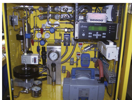
FIG. 5. The PAGES system is connected with three separate gas channels. These channels deliver gas to the sample cell.
