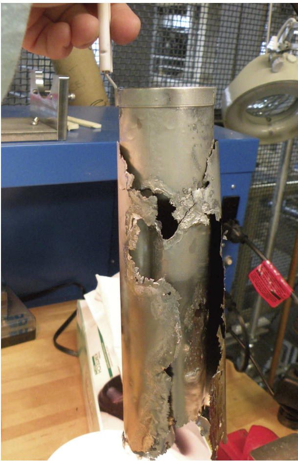
FIG. 3. Niobium embrittled by water at elevated temperature.
