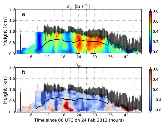
**Figure 5.** (a) Standard deviation and (b) skewness of vertical velocity. The black shading shows the location of the cloud layer, where cloud base is diagnosed from the lidar measurements and radar measurements are used to infer cloud-top height. The black line gives the lifting condensation level estimated from surface temperature and humidity measurements.
