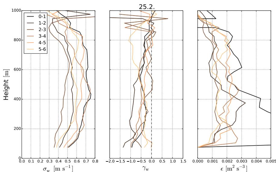
**Figure 7.** Profiles of the standard deviation ( $\sigma_w$ ) and skewness ( $\gamma_w$ ) of vertical velocity and the dissipation rate ( $\epsilon$ ) for 1 h segments during the early hours of 25 February.
