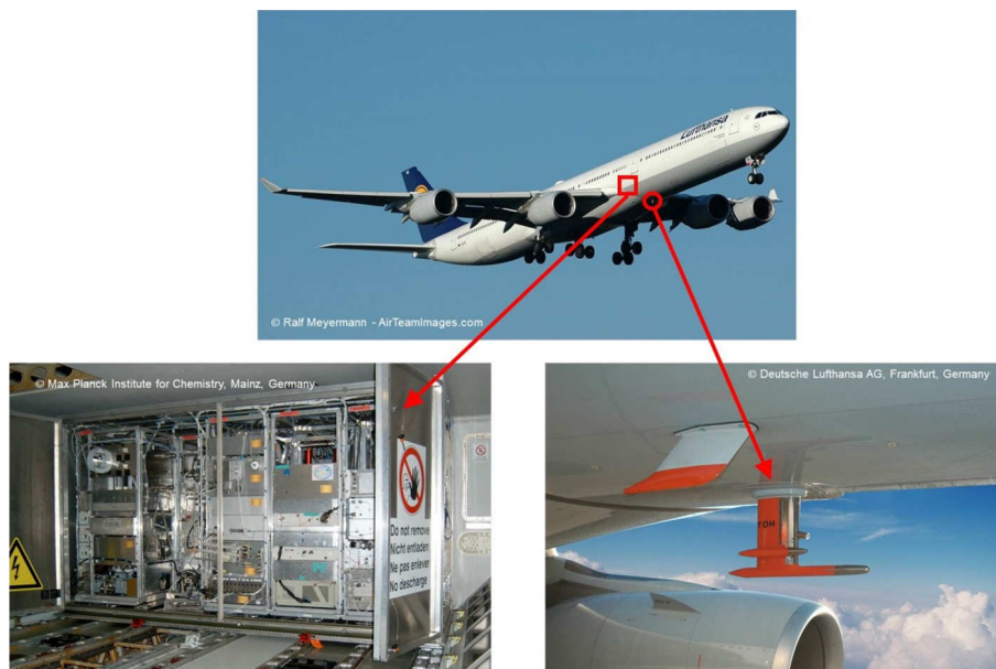
Fig. 7. IAGOS-CARIBIC aircraft, air inlet system and measurement container (Brenninkmeijer et al., 2007).
