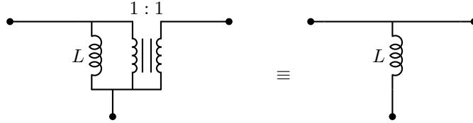
Figure 9: Circuit identity showing that inductor-ideal transformer pairs appearing in state-space Brune stages simplify in the case of turns ratio equal to one; in this case Fig. (8) becomes identical to one of the classic lossless Foster canonical forms in [10].
