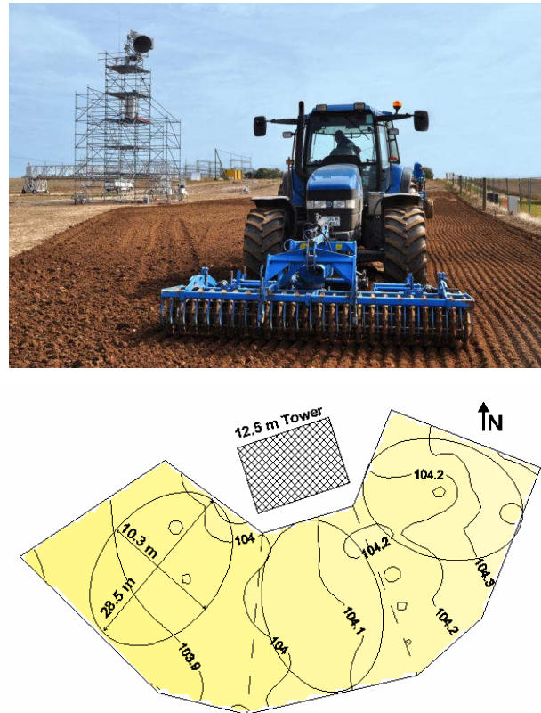
Figure IV.1 Top: mechanical field preparation (tilled plot (left from the tractor), seedbed plot (right from the tractor)). Photo from DOY 223. Bottom: location of the radiometer tower, different plots and -3 dB radiometer footprints, labeled lines and color scale denote the elevation (m.a.s.l.).
