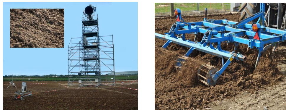
Figure III.1 L-band radiometer JULBARA and laser profiler over the plot (left). Mechanical field preparation (right).
