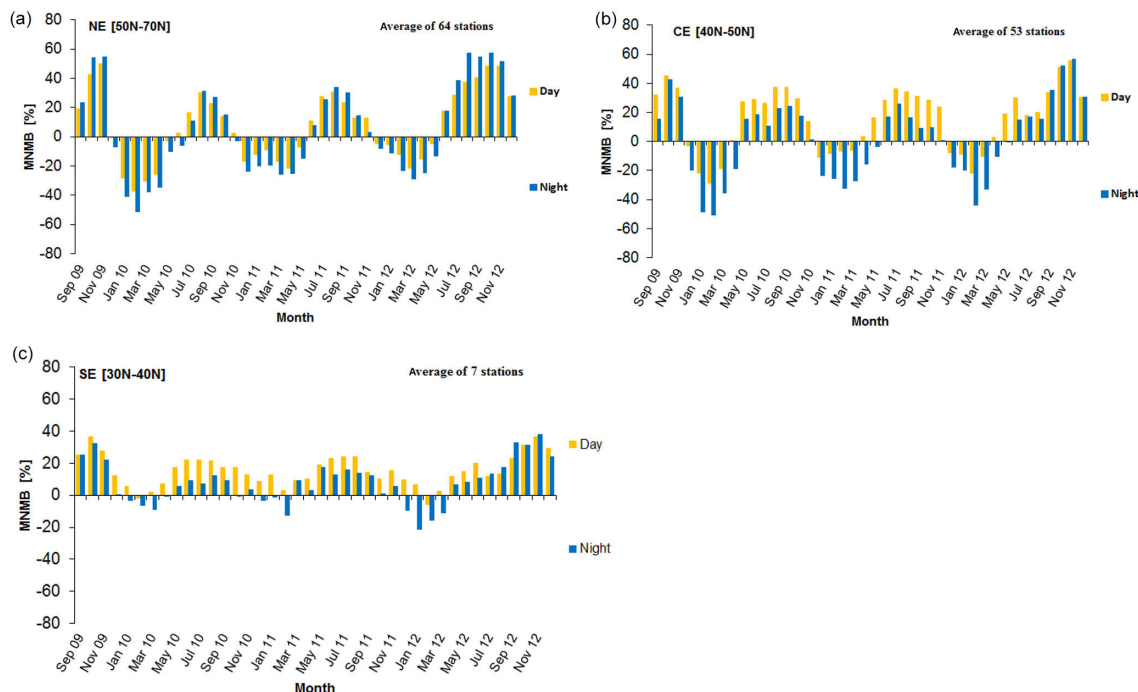
Figure 8. Modified normalised mean biases (MNMBs in %) derived from the evaluation of the MACC_ou suite with EMEP O 3 surface observations during daytime (yellow colour), and night-time (blue colour) over northern Europe (a), central Europe (b) and southern Europe (c) during the period September 2009 to December 2012.
