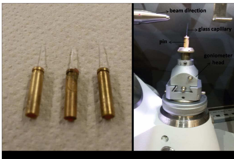
Figure 5.3(a) Metal pins with glass fibers and sample (b) goniometer head with sample mounted on the diffractometer
