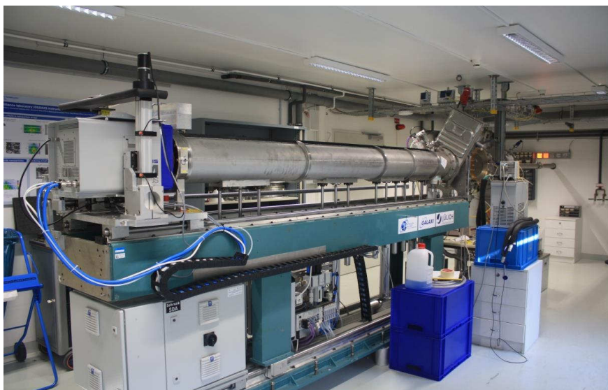
Figure 3.5: GALAXI diffractometer with sample chamber and detector.
