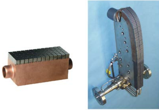
Fig. 2 (left) Monoblock from graphite (CFC) brazed on copper, as a water cooled element for the target plate, and (right) a prototype target plate module (vertical target) made from tungsten and CFC; these modules fulfill all requirements for heat exhaust under thermal cycling loads up to 23 MW/m 2 1
