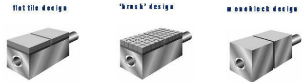
Fig. 4 Design options for actively cooled plasma facing components for divertor applications [9]
