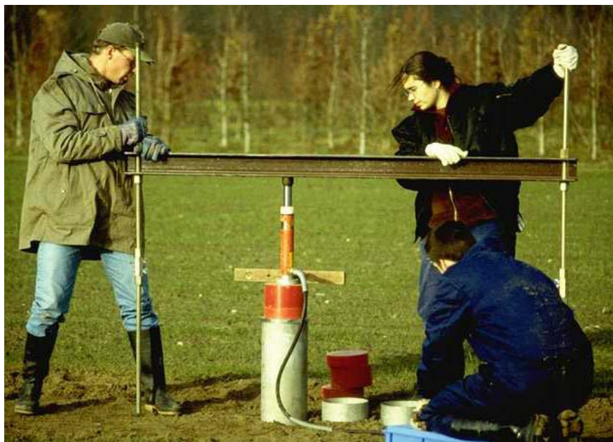
Fig. 12: Getting the undisturbed soil columns with a hand-held hydraulic ram and a T-girder abutment fixed by ground anchors in Kaldenkirchen-Hülst on 26 Nov., 1997.
