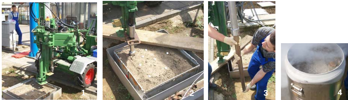
Fig. 17: Termination of the lysimeter experiment with wind tunnel: Taking soil cores with the WACKER hammer drill sampling system from Bayer, AG, Monheim, at a 0.5 m 2 lysimeter, the samples being frozen in liquid
