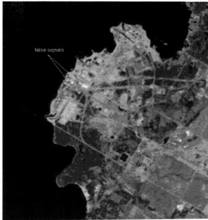
Figure 16: MAD change detection for BMS2 (August 1996 – May 1997). The first two MAD components exceeding approximately 2.2 standard deviations are in red and green. They are fused via the IHS (intensity-hue-saturation) transformation to channel 5 of the May 1997 image for better reference.
