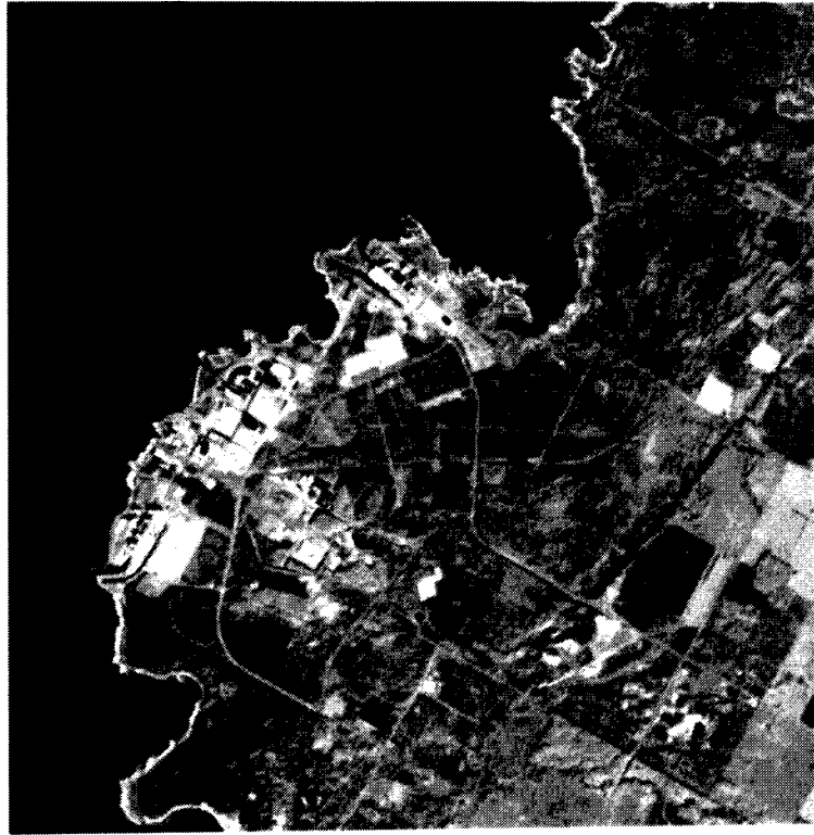
Figure 18: MAD change detection for BMS4 (August 1996 – September 1999). The first component exceeding 1.5 standard deviations is shown green. It is fused via the IHS (intensity-hue-saturation) transformation to the 15m resolution panchromatic channel of the 1999 image.
