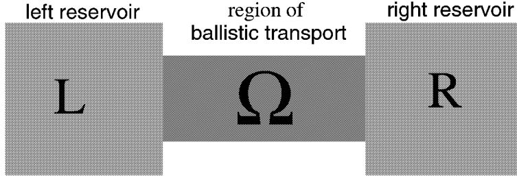
Figure 3.1: Basic setup of the Landauer approach to transport. The reservoirs are assumed to be in thermal equilibrium.
