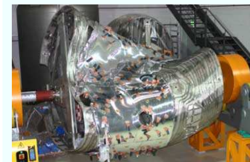
Fig. 5 Thermal insulation mounted onto one vessel half-module sector.
