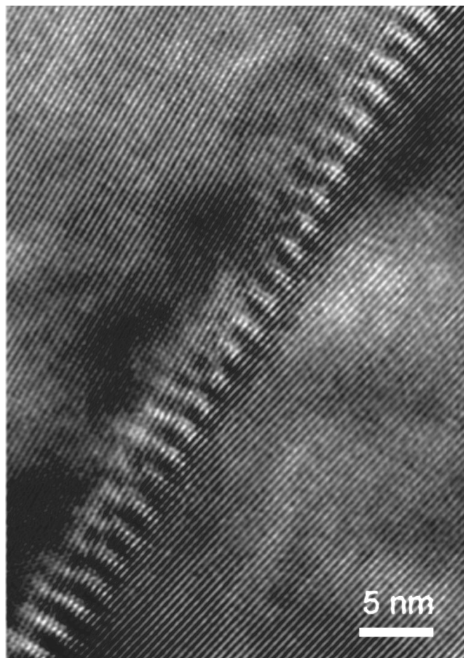
Figure 1. HRTEM of grain boundary in 1.0 mol % \text{Y}_2\text{O}_3 -doped \text{CeO}_2 . The moiré rings are also visible.
