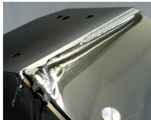
Fig.2 Photo of the tungsten plate after plasma exposure.
