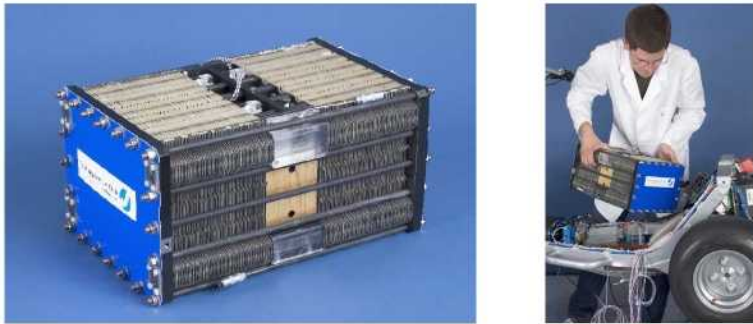
Fig. 3-2: 1.3-kW DMFC stack with integrated system (left), installation of the 1.3-kW stack in the scooter (right)
