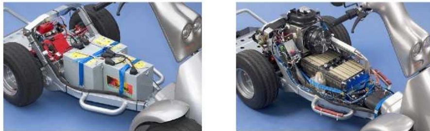
Fig. 3-4: Scooter in the as delivered state with lead-acid battery (left), after modification with DMFC system (right)
