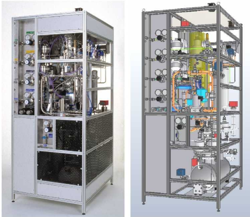
Fig. 4-10: Module for reforming kerosine, left: photograph, right: perspective sectional drawing
