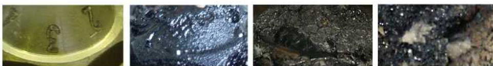
Fig. 3-15: Carbon-containing depositions in diesel reforming
