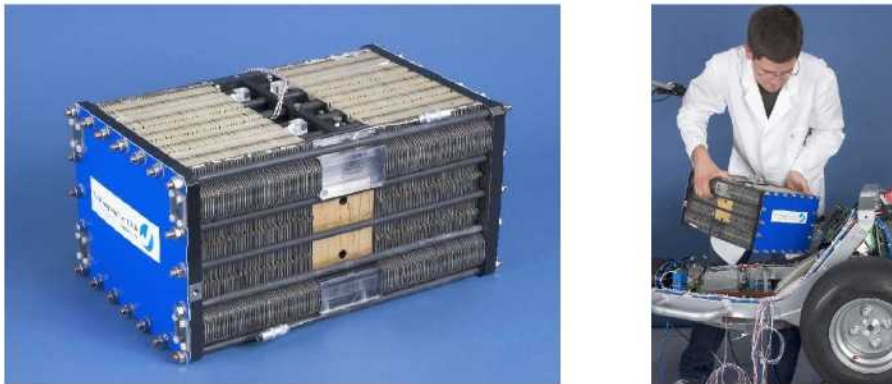
Fig. 1-3: 1.3-kW DMFC stack with integrated system (left), installation of the 1.3-kW stack in the scooter (right)
