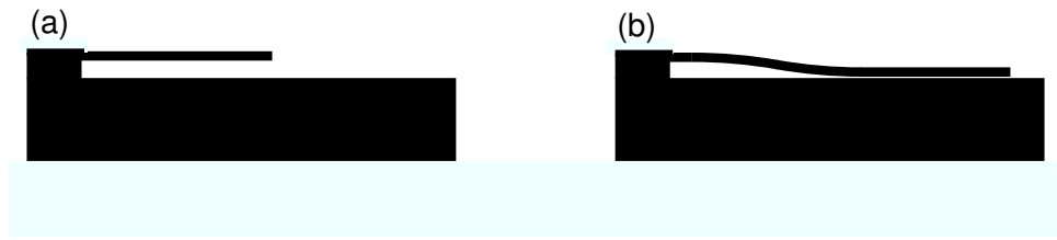
Figure 1. (a) Micrometer sized cantilever beam. (b) If the beam is too long or too thin the minimum free energy state corresponds to the beam partly bound to the substrate. Surface roughness lowers the binding energy (per unit area) and hence stabilizes the non-bonded state in (a).
