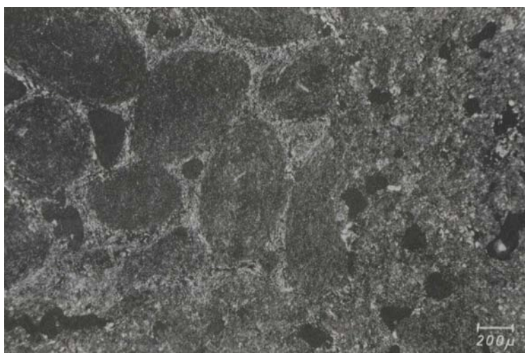
Fig. 27b Pores in Gilsonite graphite irradiated to turn-around
