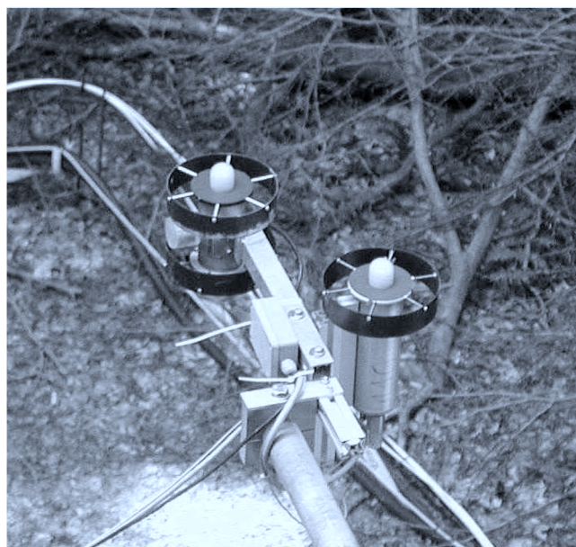
Figure 1. Setup of two filterradiometers 4 m above ground at the ECHO main tower: 4 \pi sr j(\text{NO}_2) instrument (left) and 2 \pi sr j(\text{O}^1\text{D}) instrument (right). Shadow rings (black) limited the fields of view to one hemisphere.
