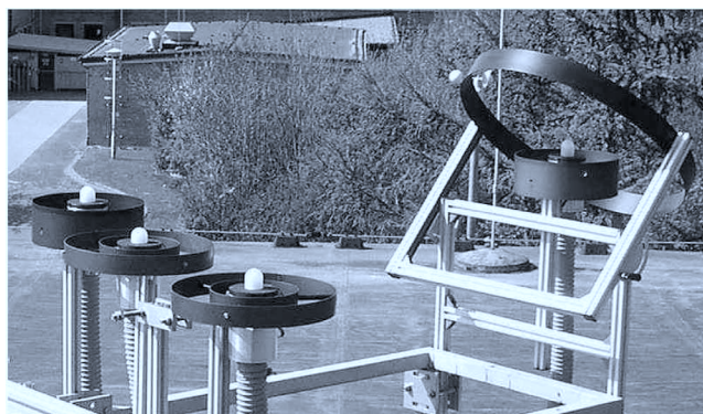
Figure 1. Spectroradiometer detector heads and shadow ring. The picture was taken at the site of the measurements above the forest before the 2003 campaign. The two heads in front belonged to the instrument that was then moved into the nearby forest.
