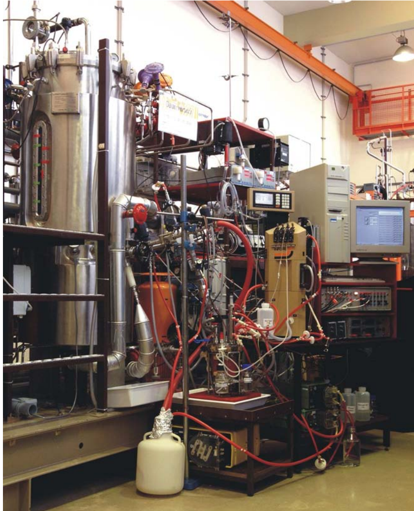
FIGURE 3.10. Experimental setup of the 1- L Sensor reactor together with the standard equipment for fermentation control and the 300- L bioreactor.
