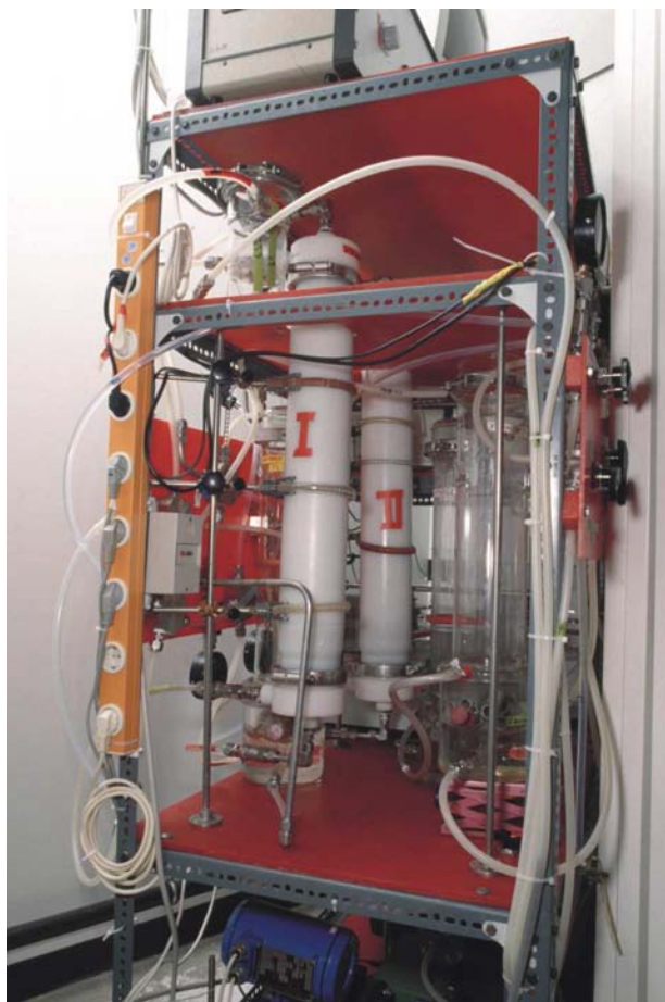
FIGURE 4.42. Experimental setup used for pilot-scale reactive extraction experiments based on two LiquiCell TM hollow fiber modules for extraction and back extraction, respectively.
