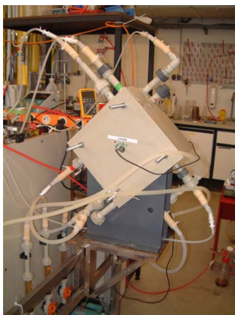
FIGURE 5.10. Electrodialysis cell (four stacks) used for the separation of pyruvic acid.
