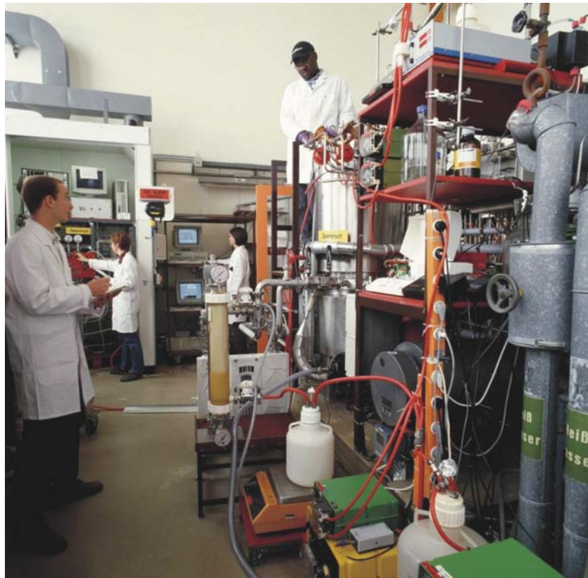
FIGURE 4.47. Picture of the total pilot-scale ISPR setup used of on-line L-Phe separation using reactive extraction. The 300-L bioreactor is shown together with the by-pass consisting of a peristaltic pump and the ultrafiltration unit. On the bottom, the red tubes are identifiable which connected the bioreactor with the reactive-extraction system (in the background). Also via the red tubes, the L-Phe reduced permeate stream is recycled into the bioreactor. A corresponding movie is offered at the internet at www.fz-juelich.de/ibt/ferm .
