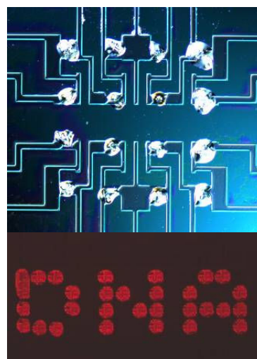
Fig 3.19 Image of Cy3-labelled ssDNA spotted on the transistor gates with the aligned microspotting system. The volume of the droplets was calculated to approximately 65pl
