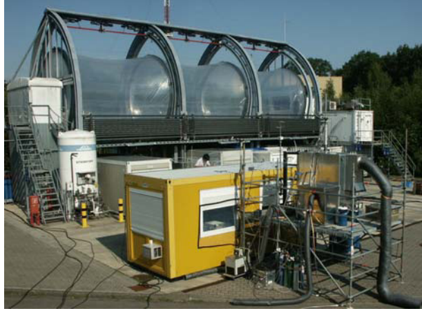
Figure 6.1: Atmosphere simulation chamber SAPHIR with opened shutter system. The “MobiLIF” system can be seen on the scaffold (HOxComp campaign in July 2005).
