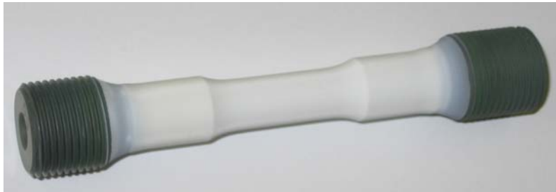
Figure 4.1: Experimental TMF sample.
