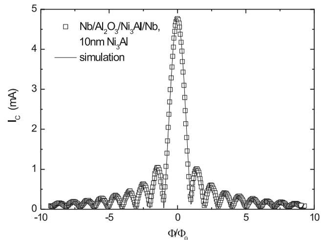
FIG. 2. Fraunhofer pattern of a typical circular Nb/Al/Al<sub>2</sub>O<sub>3</sub>/Ni<sub>3</sub>Al/Nb Josephson junction, measured at 4.2 K (rectangles). The junction size is about  $1000 \mu\text{m}^2$ . The solid line results from a fit to the Fraunhofer function.
