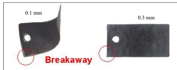
Figure 6.7: Macro images of specimens with different initial thicknesses (steel Crofer A) after cyclic oxidation at 900°C in air showing breakaway and deformation of the specimens after oxidation
