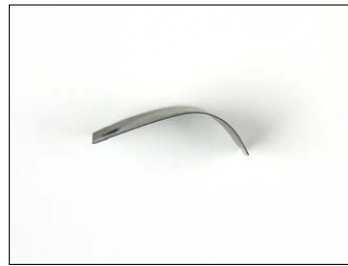
Figure 6.6: Macro image of specimen with 0.1 mm initial thickness (steel Crofer A) after 1000 h cyclic oxidation at 800°C in air showing deformation of the specimen after oxidation
