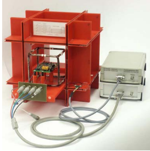
Figure 3.7: Measurement setup for sensor sensitivity determination, after Zimmermann et al., 2005
