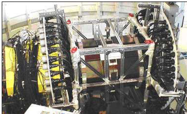
Fig. 9. A photograph of the ENSTAR detector mounted at the COSY beam line along with its support structure and the stand which has been used to transport the detector to the beam line.
