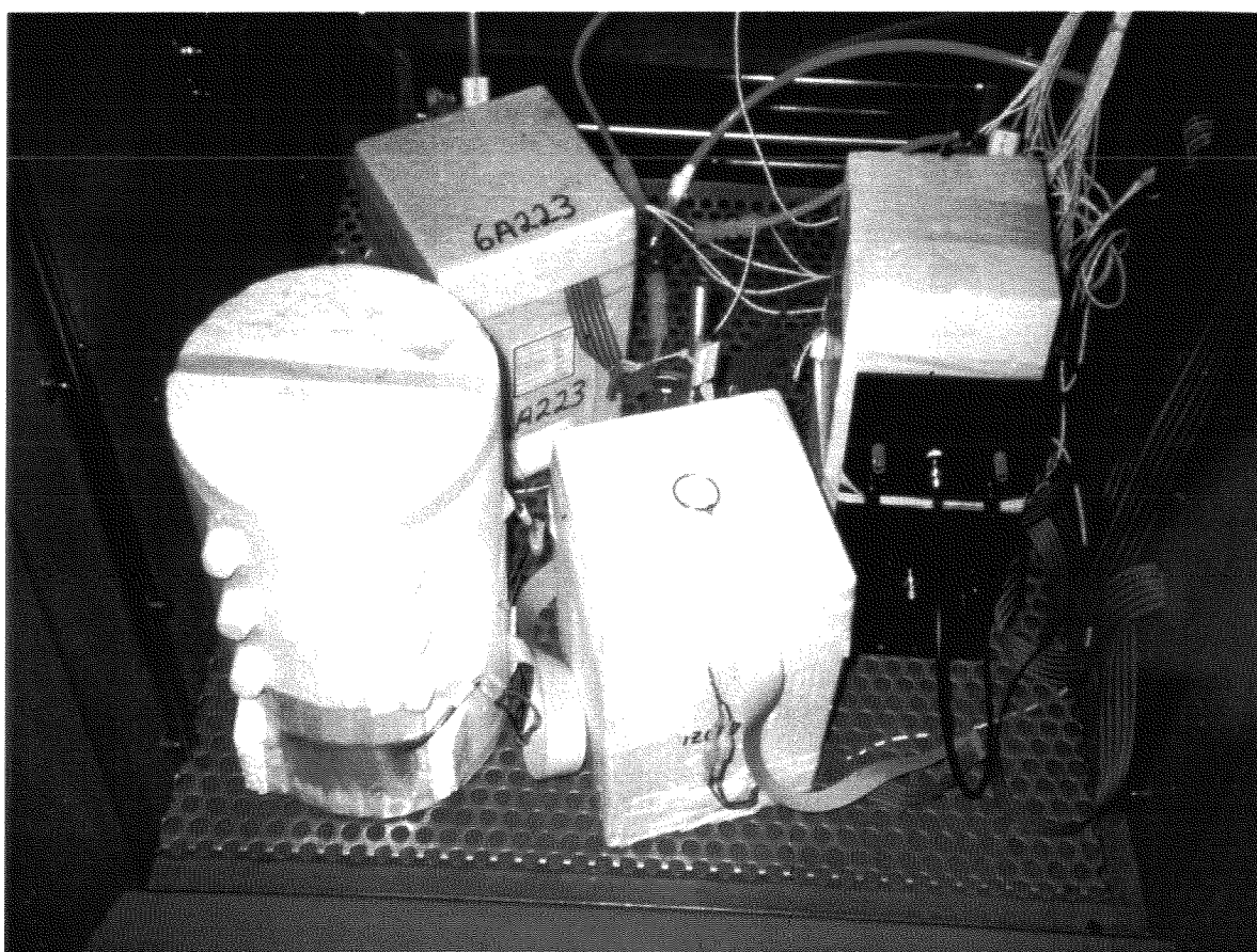
Figure 13: Four different ozone sondes installed in the environmental simulation chamber just prior to a simulation of an ozone sounding during JOSIE-1996
