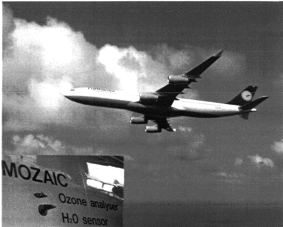
Figure 17: Airbus A340 equipped with MOZAIC-Humidity Device. Inlet system mounted at the outside skin of the aircraft close to the cone.
