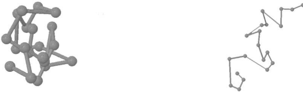
Figure 4: On the left is shown a typical conformation at temperature T = 0.5 . Conformations at lower temperatures are of a globular structure. The right picture shows a conformation at temperature T = 1.5 . For higher temperatures this polymer forms coil-like structures.
