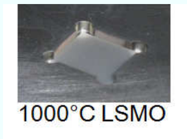
(c) LSMO/STO: After preparation, deposited LSMO shows color expected for 20nm thin film, while STO corners without deposited LSMO are white indicating no oxygen deficiencies
