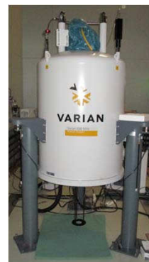
Fig. 51: A Varian 600/54 MHz premium shielded high resolution spectrometer (14.1 Tesla; Magic angle 54.7°) used for the MAS-NMR measurements shown in the next section.
