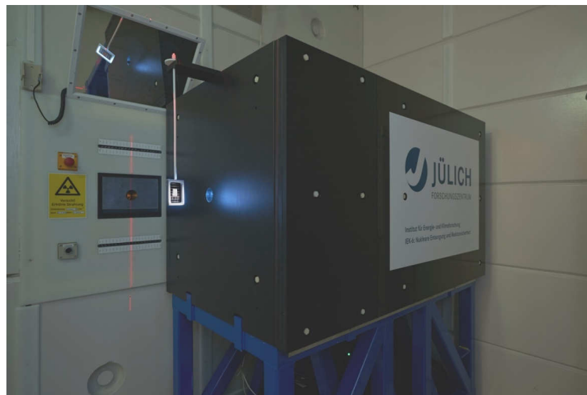
Fig. 74: FaNGaS, the Fast Neutron Gamma Spectroscopy instrument at the SR10 beam line of the FRM II Research Reactor in Garching.
