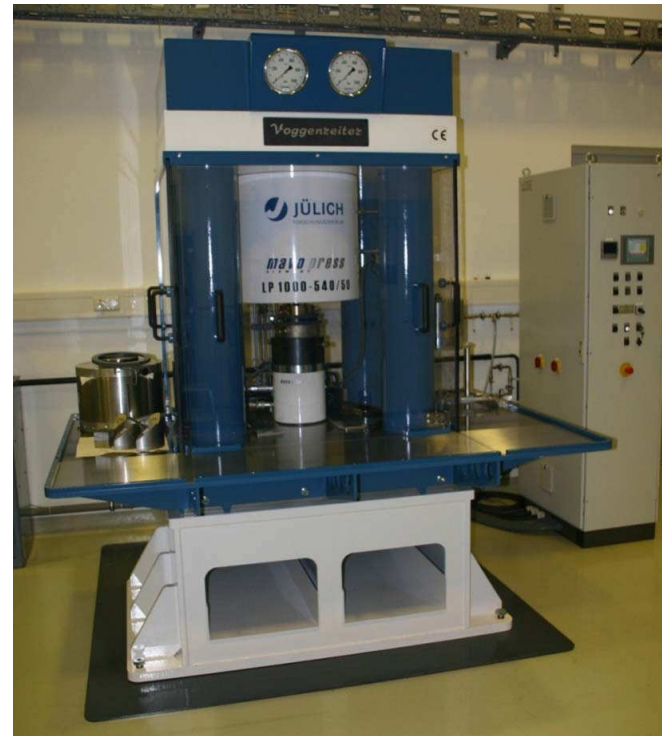
Fig. 12: Combined piston cylinder / multi anvil press. In this picture the piston cylinder module is installed under the main cylinder. On the left workbench side of the device the walker-type multi anvil module is visible.
