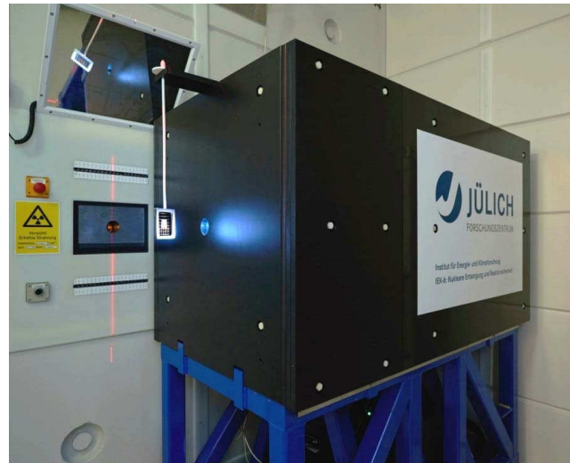
Fig. 8: Fast Neutron Gamma Spectroscopy (FaNGaS) instrument installed at the FRM II.
