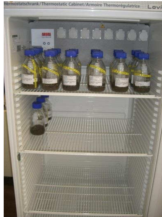
Figure A2: Thermostat Incubator for Degradation Experiment ( \sim 25^{\circ}\text{C} ).
