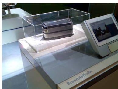
Figure 18. Volkswagen high-temperature fuel cell (photo taken at the Hanover Trade Fair, 2007).
