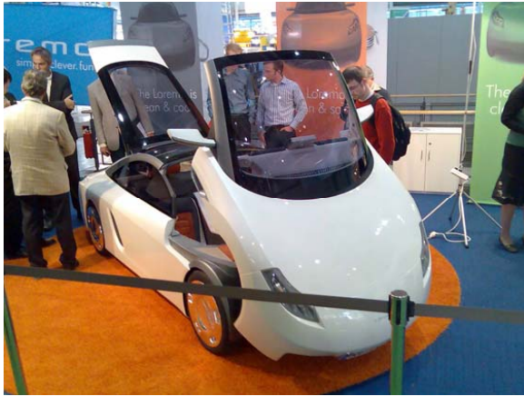
Figure 15. Lightweight materials. (Simple engineering with today's available innovations allowed Loremo to construct a car with a fuel consumption of only 1.5 litres of fuel per 100 kilometres 29 . It is powered by a 2 cylinder turbo diesel engine.)
