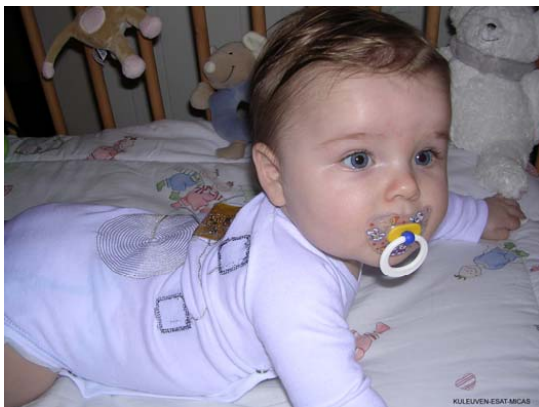
Figure 38. Paediatric application of a wireless monitoring suit (photo with kind permission of K.U. Leuven)
