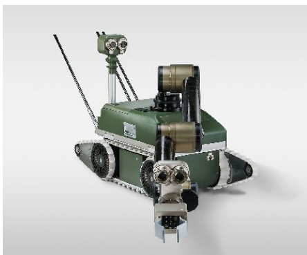
Figure 27. Robot for NBRC detection and mitigation of ammunition (photo from Diehl Stiftung & Co. KG)
