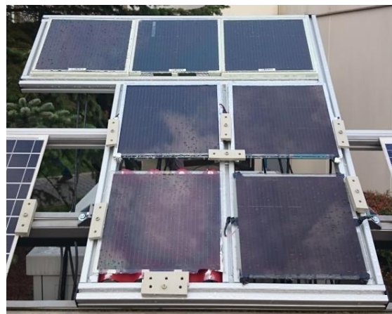
Figure 1: Photographs of solar modules on thermal insulating building materials (left) and the modules under consideration on the outdoor measurement setup (right).
