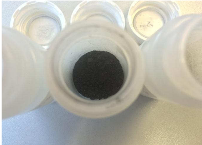
Figure 12. Polycrystalline Sample of the \text{Mn}_{5-x}\text{Fe}_x\text{Si}_3 Series produced by cold crucible melting after the grinding process.
