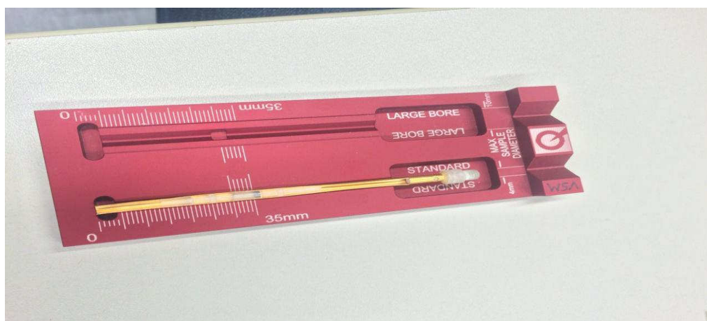
Figure 13. Mounting station to center the polypropylene sample holder with the sample at the correct position.
