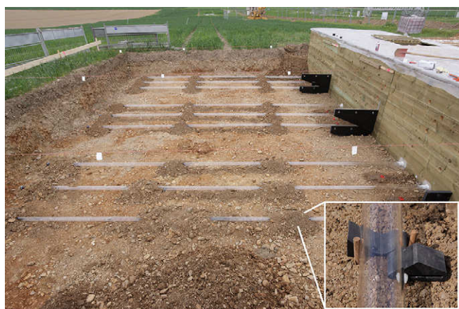
Fig. 1. Installation of the minirhizotron facility in the upper part of the test site. The wood container is the accessible facility. Wedge-shaped fixture blocks shown in the right corner were used to fix the tubes during soil backfill.
