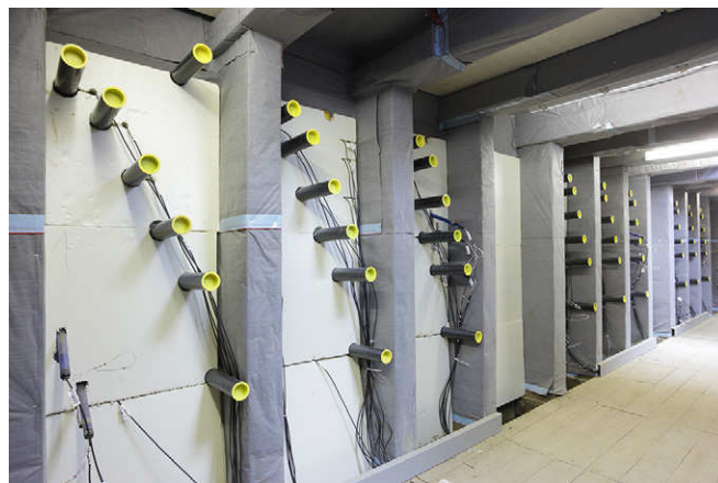
Fig. 2. Interior view of the minirhizotron facility. The rhizotubes were installed perpendicular to the wall profile.
