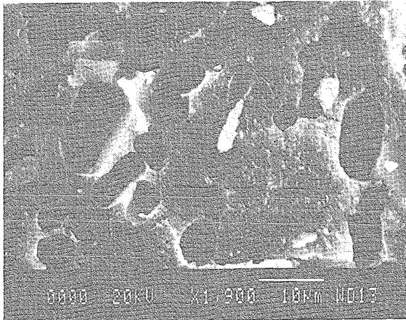
Figure 6: SEM image of large pores in sample GP4
