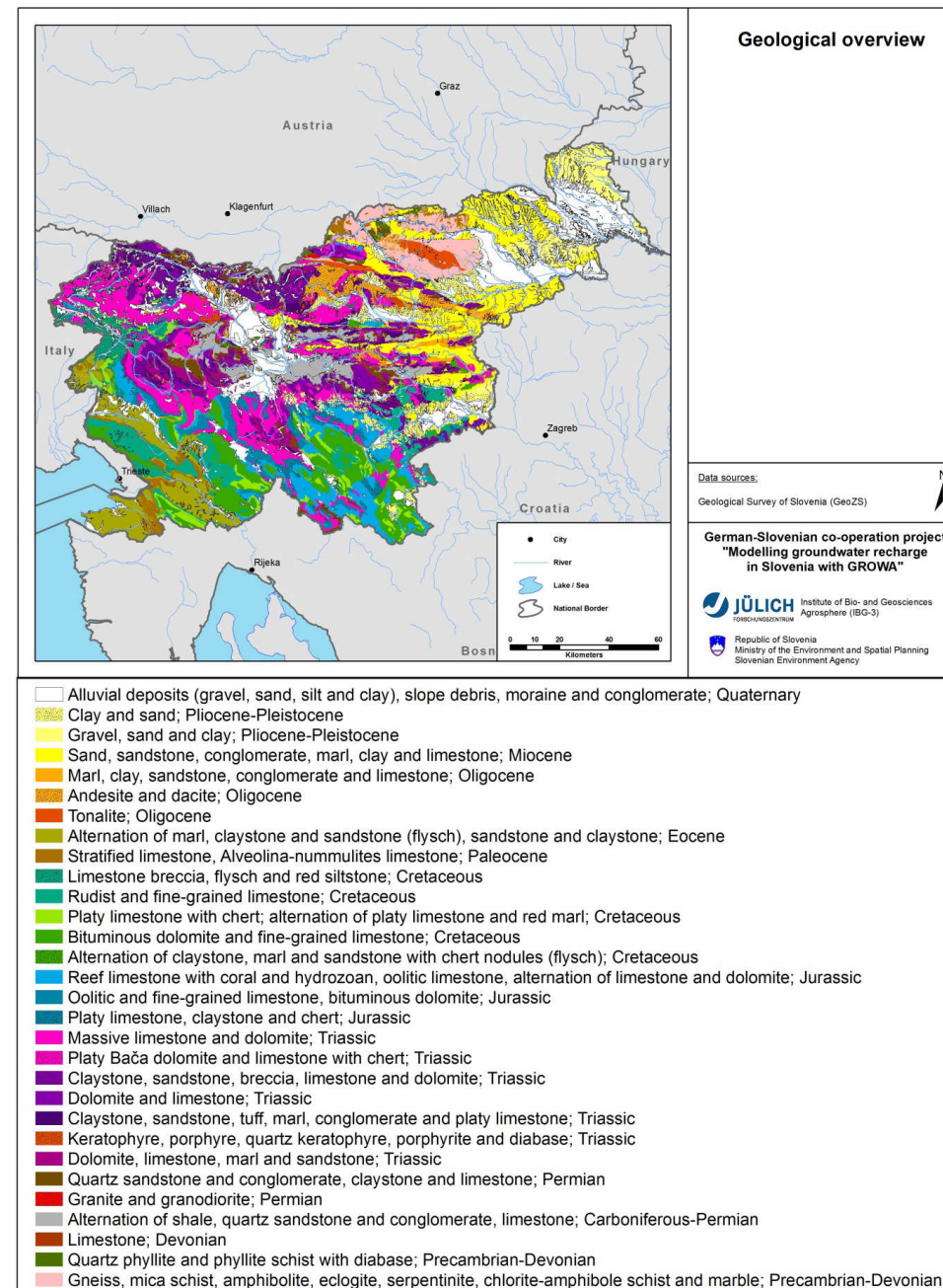
Figure 3-14: Geological overview of Slovenia, compiled from basic geological map of SFRJ 1:100,000 (OGK1, 1967-1998) and basic geological map of Slovenia 1:250,000 (Buser, 2010).
