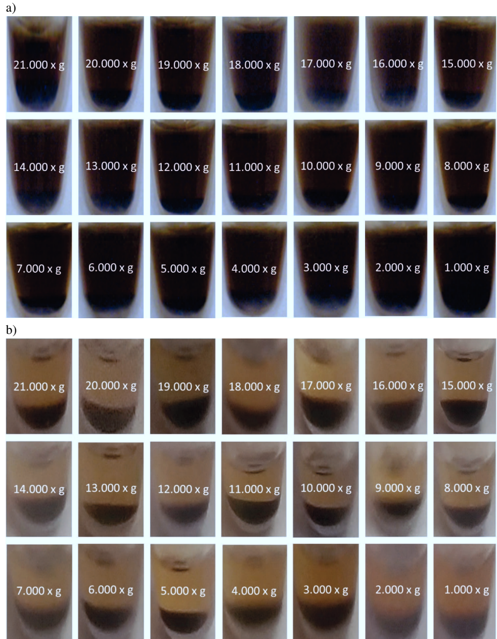
Figure 5.8: Nanoparticle sedimentation after 2 h of centrifugation at 10 °C for different accelerations, a) batch O1, b) batch O2.
