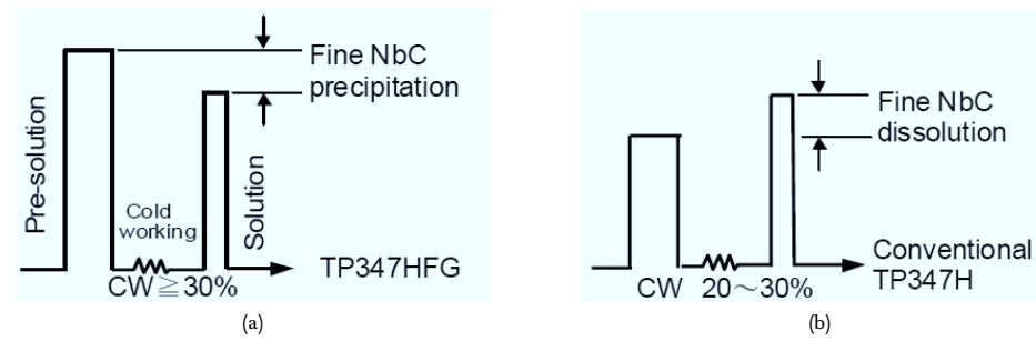
Figure 2.28: Thermomechanical treatment of an 18Cr-12Ni-Nb steel, (a) the novel TP347HFG, and (b) the standard TP347H [14]
