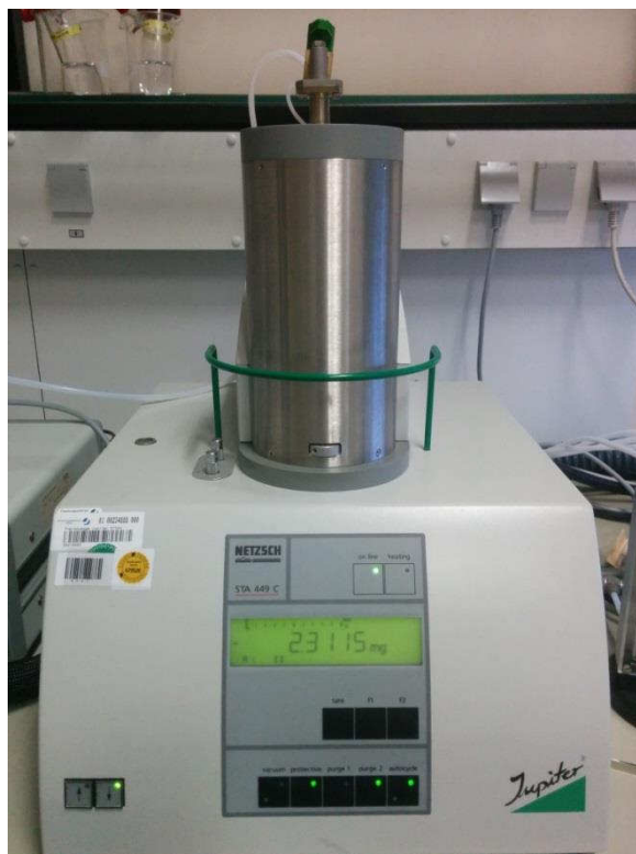
Figure 2.10: Netzsch STA 449C Jupiter apparatus for TG- DCS experiment
