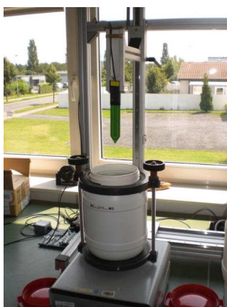
Figure 3. The container with glass beads (M2) on top of the vibration machine.
