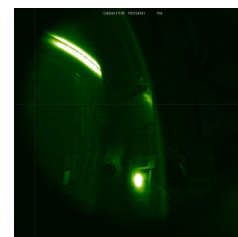
FIG. 8. CIII emission at limiter in module 5 (double-stripe structure at top left) detected with a visible camera and an interference filter at 467 \pm 5\ \text{nm} . The bright spot at bottom right is due to NeI emission from neon injected by the helium beam injection system for edge cooling experiments.
