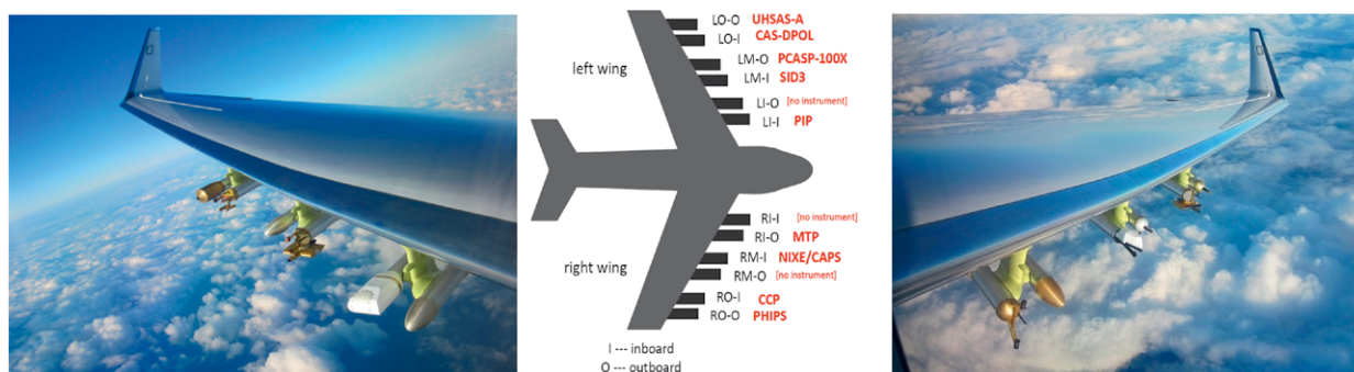
FIG. 1. Particle-measuring systems in HALO wing stations: six cloud probes, two aerosol spectrometers, and a microwave temperature profiler were integrated in the wing stations. Details of the instruments are given in Table 1.
