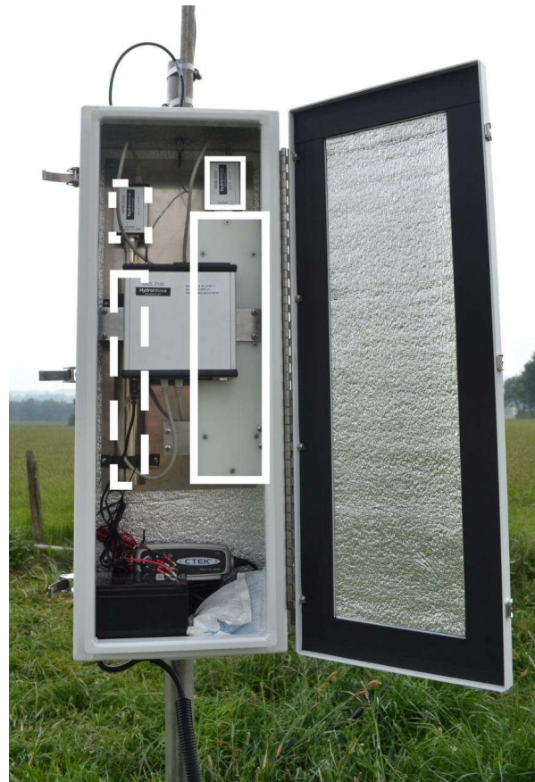
Figure 4: Cosmic-ray probe located at the test site Rollesbroich is shown with the slow (white, dashed) and fast (white) neutron counter with the pulse modules on top.
