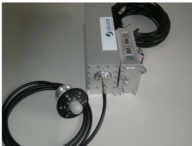
Figure 1. Basic components of a CCD array spectroradiometer system for airborne measurements. Receiver optics with optical fiber (black, front), spectrometer including monochromator and CCD array detector (middle), and cooling electronics (right).
