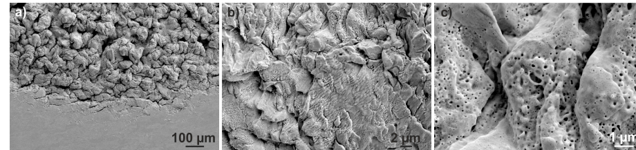
Figure 4.37: The SEM images illustrate the exposed surface of a T sample after 100,000 transient thermal events. Pronounced plastic deformation occurred due to the high number of repetitive stress cycles and a helium induced spongy morphology was detected.
