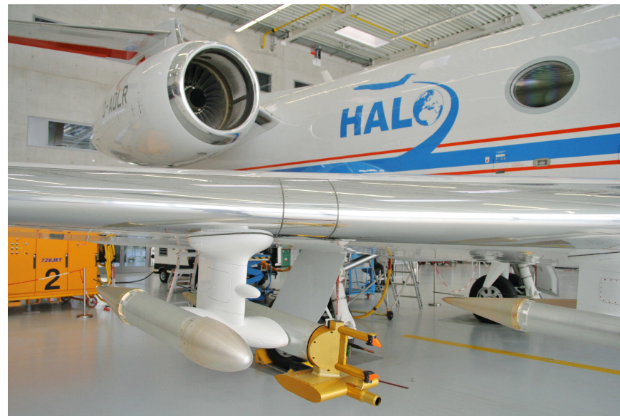
Figure 2.2: NIXE-CAPS mounted on HALO.
